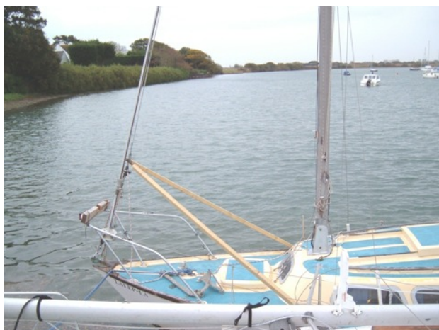
Simple 'A' frame made from two pieces of 2x2 (inches) ready to use.
