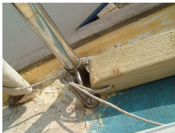
The aft end is rounded to allow rotation during lifting and tied to the stanchion base.
