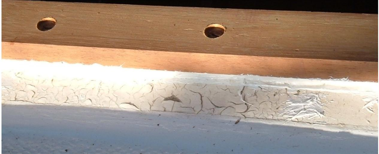
Finally a second piece of wood was fitted just behind the first which the washboard sits on and is about 8 mm lower. This provides a step and ensures that the water drains into the cockpit and not the cabin. Note that the original was just a single piece of wood, but the profile would have been difficult to reproduce.
