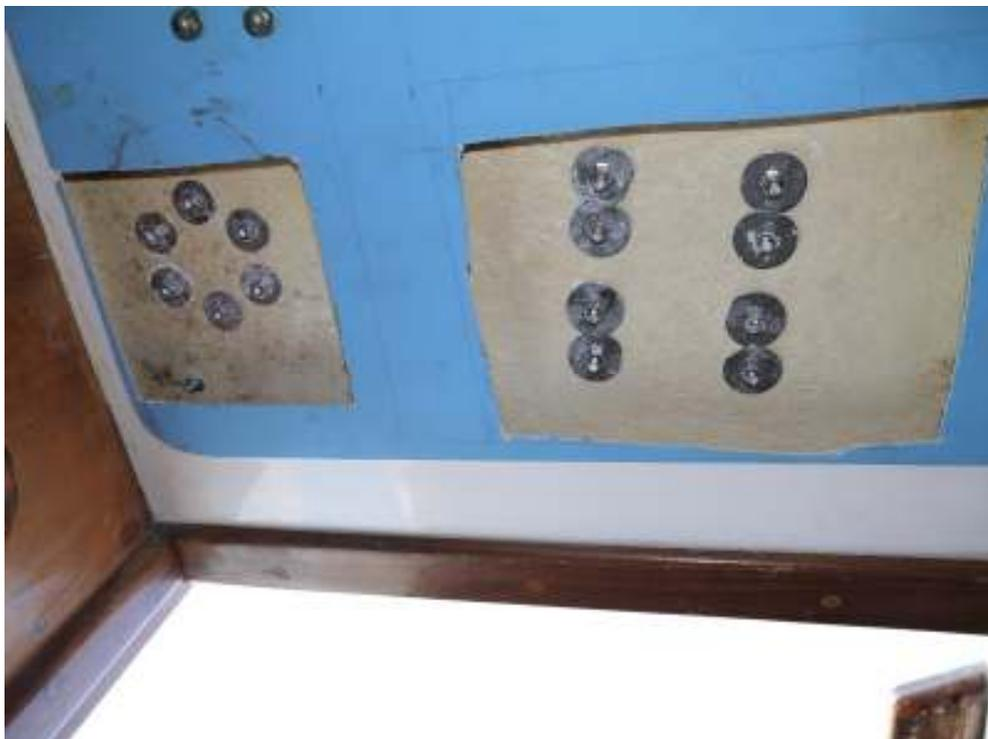
*Winch bolts and, visible at the top, the bolts securing the K Cam cleat.*
