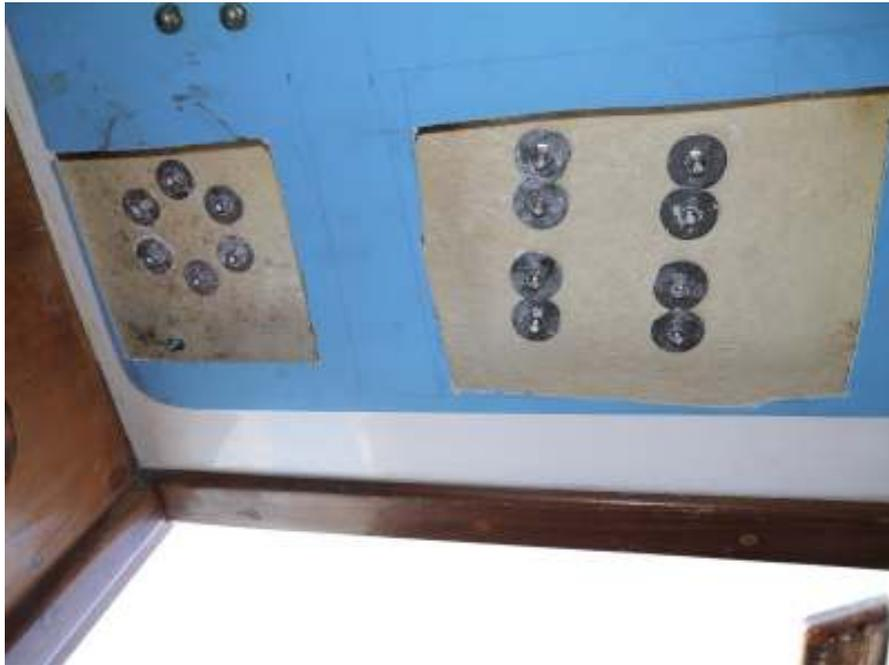
*Securing points of the two double rope clutches (right) and the Harken winch.
