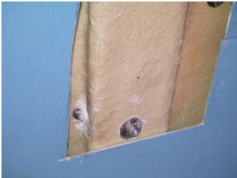
*The aft bolt of the port-side deck organiser has come through too close to the supporting beam making it impossible to use a washer!*
